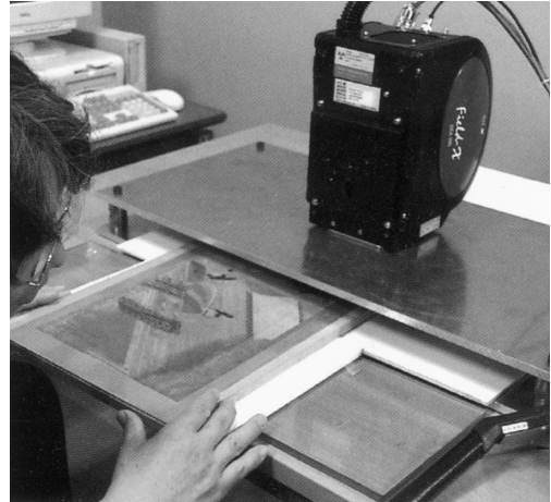
FIGURE 2. A portable x-ray machine being used to scan the handscroll painting, from the "Yomigaeru Genji monogatari emaki " exhibition catalog. Photograph courtesy of Japan Broadcasting Corporation, Tokyo.
